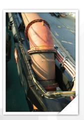
It is about the manufacture of bimetallic wear parts, generally tubes, when the inside layer requires a resistance to high abrasion and the outside layer a strong mechanical resistance to shocks.
